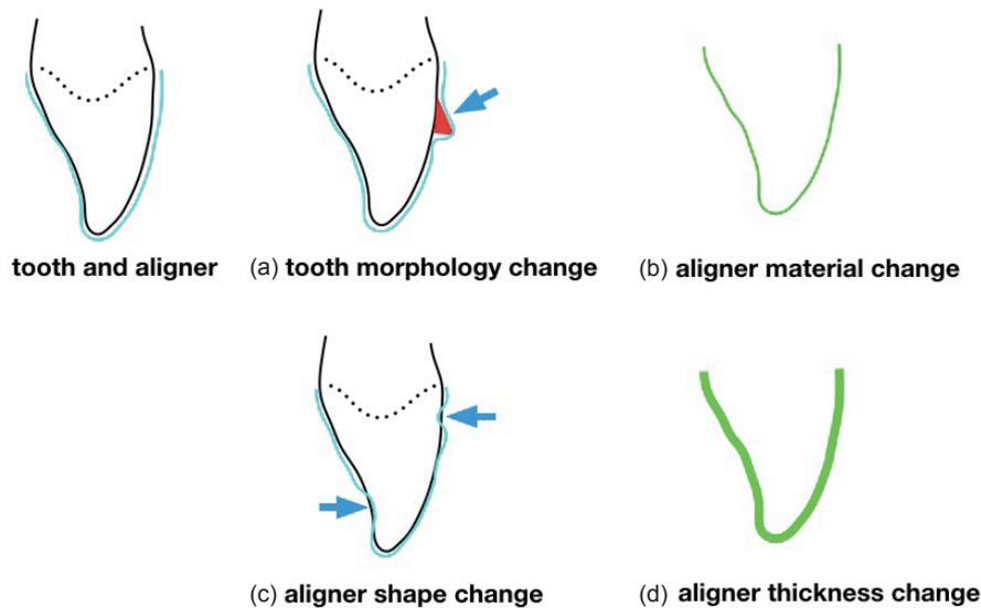
**Figure 2.** Controlling force generated by interaction of tooth morphology (a) and aligners modifications (b, c, d) .
